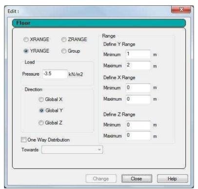
Figure IV-3 input window of floor load generator
